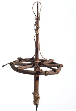
A pirori (cord drill), used by Māori to create holes in weapons, adornments, etcetera. xl
