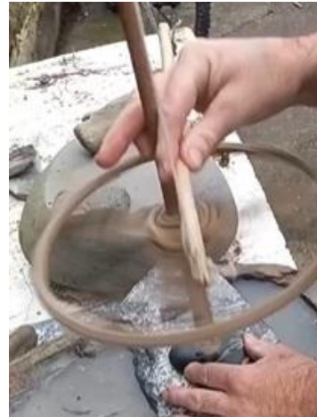
A pirori (cord drill), used by Māori to create holes in weapons, adornments, etcetera. xl
